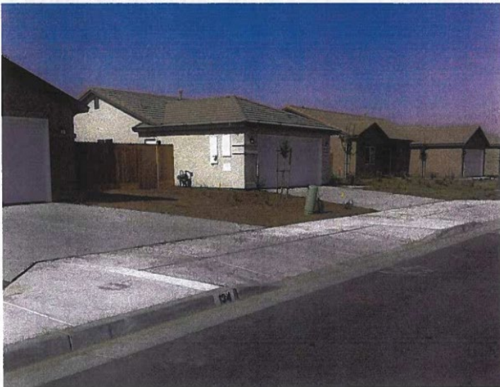
Driveways without rolled curb & gutter
